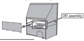
Using an open-end or socket 7/16" wrench, unfasten the 14 bolts located inside the cabinet, where the top and bottom portion of the cabinet meet.
